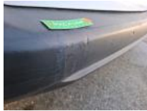
Coin pare-chocs ARG, Griffes(s), Acceptable
