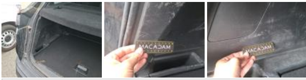
Garnit. int D coffre, Griffe(s), Acceptable
