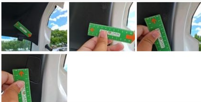
Garnit. zone de chargement, Griffe(s), Acceptable
