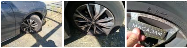
Jante alum. ARD bi-ton/polychrome, Griffe(s), E - Remplacer
