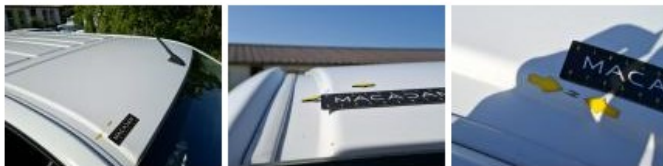
Pavillon cabine, Bosse(s) et griffe(s), Acceptable
