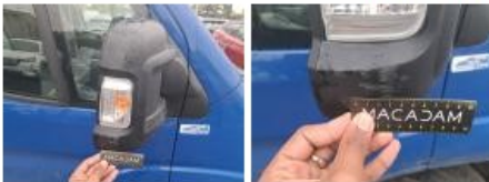
Outside rear-view mirror housing R, Scratch(es), Repair/replace (lump sum)
