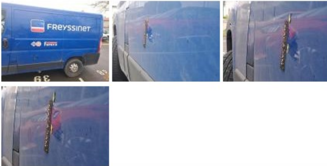
Car body corner RL, Dent(s), Repair and paint (complete)
