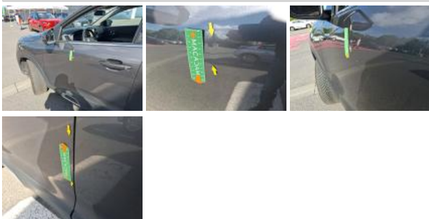
Porte ARG, Griffe(s), Acceptable
