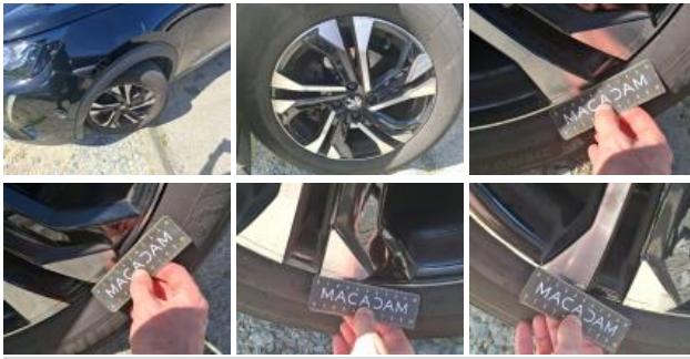
Jante alum. ARG bi-ton/polychrome, Griffe(s), E - Remplacer
