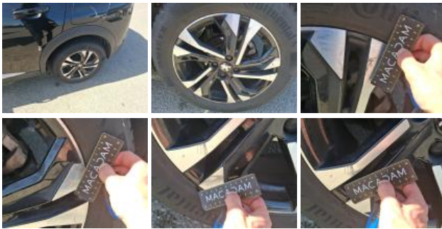
Jante alum. ARD bi-ton/polychrome, Griffe(s), E - Remplacer
