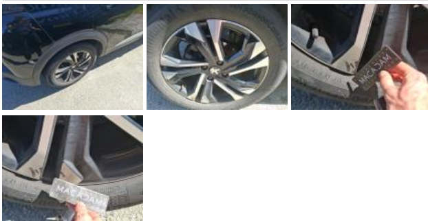
Jante alum. AVD bi-ton/polychrome, Griffe(s), E - Remplacer
