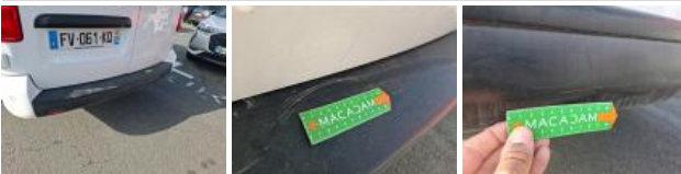
Coin pare-chocs ARG, Griffe(s), Acceptable
