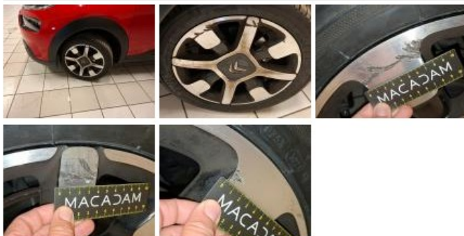
Jante alum. AVG bi-ton/polychrome, Griffe(s), E - Remplacer
