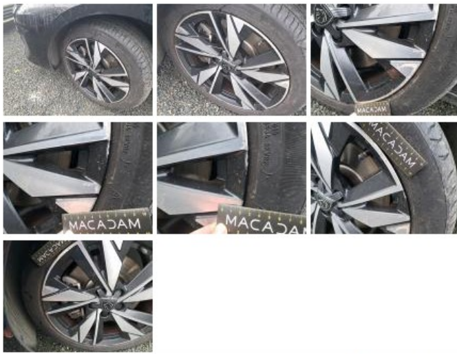
Jante alum. ARG bi-ton/polychrome, Griffe(s), E - Remplacer
