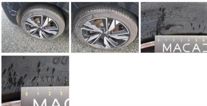
Jante alum. AVD bi-ton/polychrome, Griffe(s), E - Remplacer
