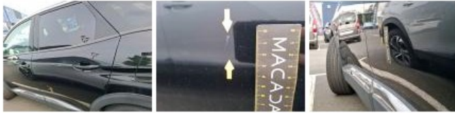
Aile ARG, Bosse(s) et griffe(s), Acceptable
