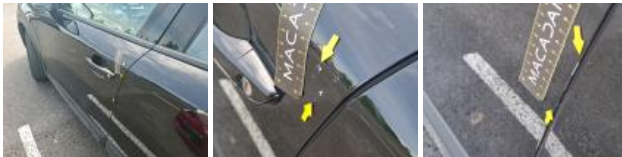
Porte ARG, Griffe(s), Acceptable
