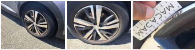
Jante alum. AVD bi-ton/polychrome, Griffe(s), E - Remplacer
