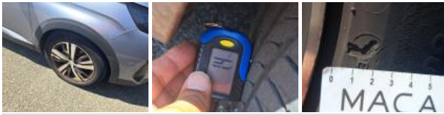
Jante alum. AVD bi-ton/polychrome, Griffe(s), E - Remplacer
