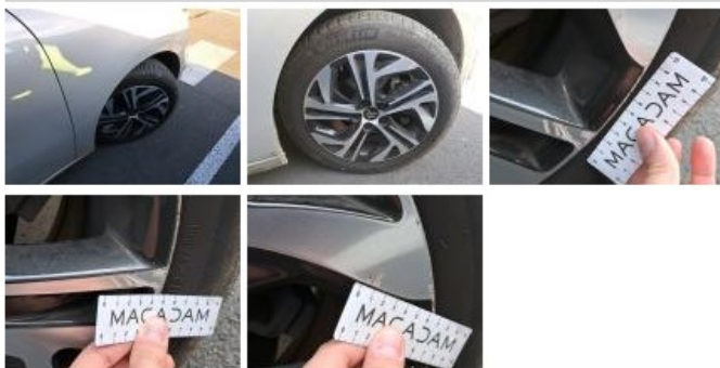
Jante alum. ARD bi-ton/polychrome, Griffe(s), E - Remplacer
