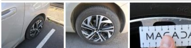
Jante alum. AVG bi-ton/polychrome, Griffe(s), E - Remplacer
