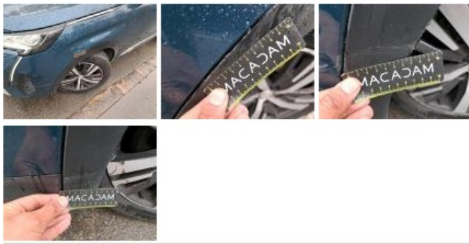
Aile ARG, Bosse(s) et griffe(s), Acceptable
