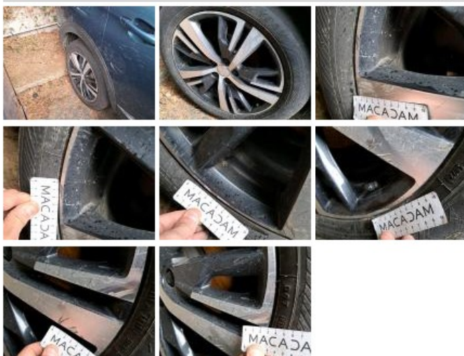
Jante alu AVD bi-ton/polychrome, Griffe(s), E - Remplacer
